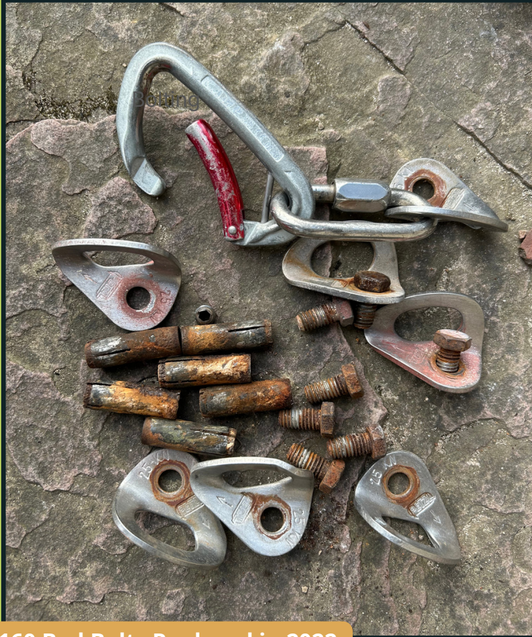
160 Bad Bolts Replaced in 2022.
